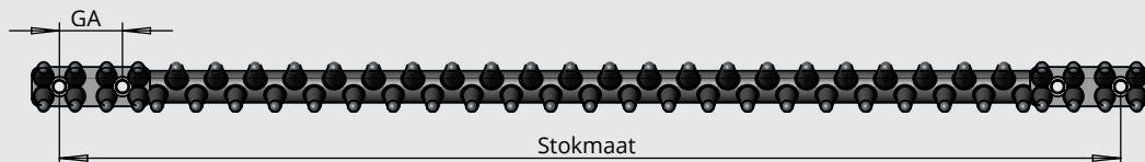
In determining the correct width of the sieve web, it is important that the rods have the correct "stokmaat". This is the distance between the two outside rivet holes, C.T.C. When ordering loose rods it is important that you mention the stokmaat as well as the distance between the holes in one end.
