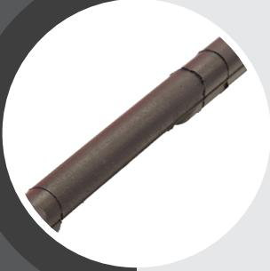
To protect the product from damage, we can vulcanize a soft rubber layer onto the rods. This rubber has a hardness of 30-35° shore. Because the rod is vulcanized over the total length, including the flattenings, this offers optimal protection. With these rods, the centre belt is attached with OGP. Because each rod must be vulcanized in a mold not every width is available.
