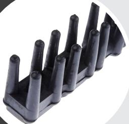
This is a ø10mm rod, on which 2 rows of rubber fingers are vulcanized in a U shape. Compared to the V10 profile, the rubber fingers are vulcanized to the sides of the rod instead of on the top. These fingers are approximately 25mm high and asymmetrically placed, also 20mm from each other. A U-profile hedgehog web has the advantage of having sieve capacity. This profile is not available in every width.
