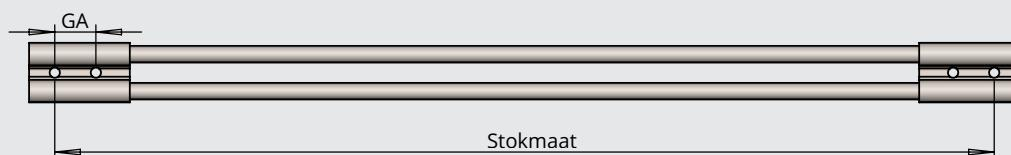
In determining the correct width of the sieve web, it is important that the twin rods have the correct "stokmaat". This is the distance between the two outside rivet holes, C.T.C. When ordering loose twin rods it is important that you mention the stokmaat as well as the distance between the holes in one end. Without further notice, we assume this distance to be 20mm in 50mm wide traction belts and 32mm in 60 or 75mm wide traction belts. On request we can also make these distances 24 or 30mm.
