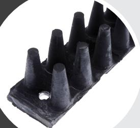
This is a flat steel profile, 4x30mm, on which 2 rows of rubber fingers are vulcanized. These fingers are 30mm high and are also placed C.T.C. 20mm from each other. P30 rods are usually riveted to traction belts with a pitch of 40mm.
