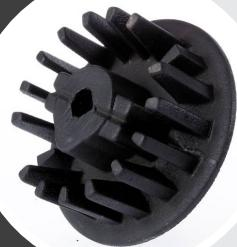
Sprockets type N are suitable for driving high cam belts. These sprockets give a secure drive, without wear on the rods of the sieve web. Sprockets type N can be supplied without a flange, so that they can be assembled to drive the centre belt.
