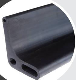
To transport the product at steep angles we have rubber flights (RM) in 9 different heights. Because of the functional design of these flights they can be assembled to every pitch. When the flight is not fitted tightly between the traction belts, its back will be cut out to fit a cable grip. This prevents the flight from moving sideways.
