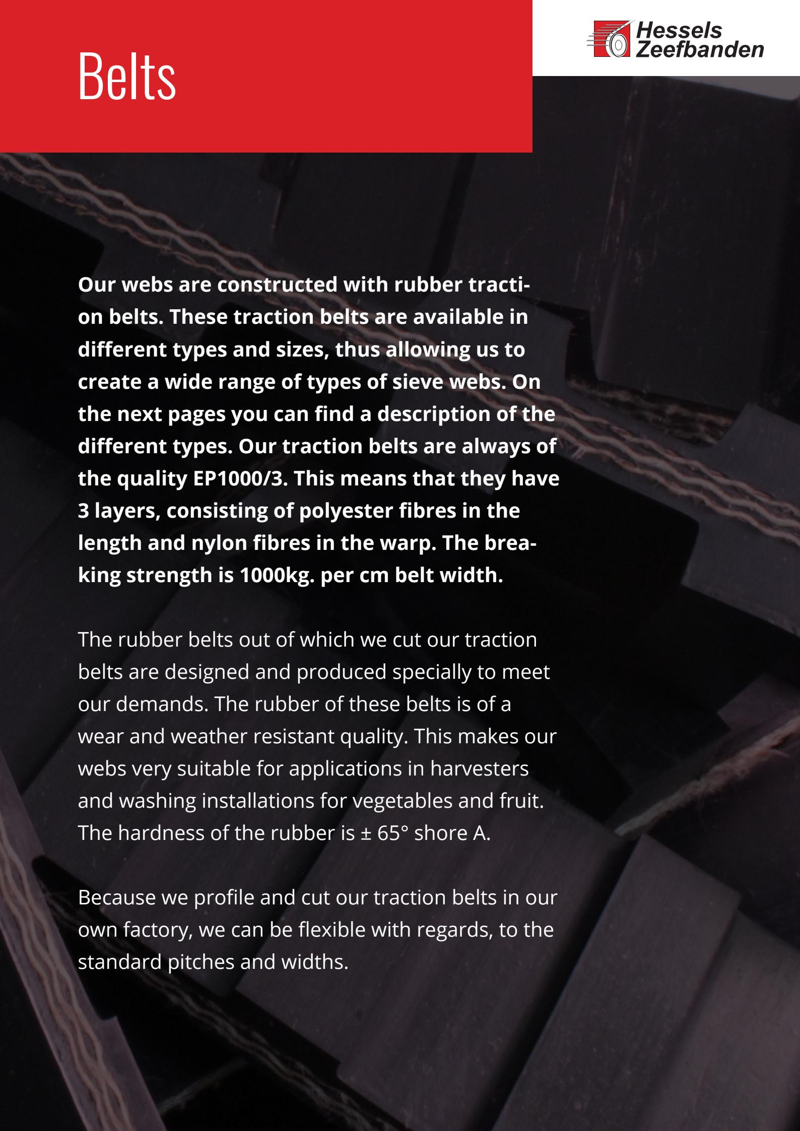
**Our webs are constructed with rubber traction belts. These traction belts are available in different types and sizes, thus allowing us to create a wide range of types of sieve webs. On the next pages you can find a description of the different types. Our traction belts are always of the quality EP1000/3. This means that they have 3 layers, consisting of polyester fibres in the length and nylon fibres in the warp. The breaking strength is 1000kg. per cm belt width.**
