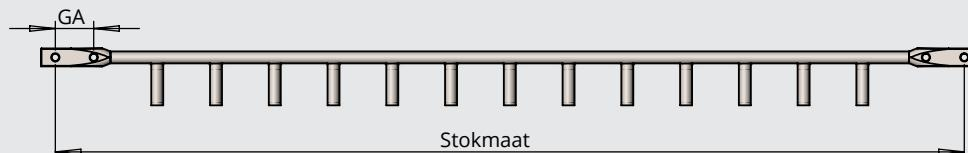
In determining the correct width of the sieve web, it is important that the rods have the correct "stokmaat". This is the distance between the two outside rivet holes, C.T.C. When ordering loose rivet rods it is important that you mention the stokmaat as well as the distance between the holes in one end. Without further notice, we assume this distance to be 20mm in 50mm wide traction belts and 32mm in 60 or 75mm wide traction belts. On request we can also make these distances 24 or 30mm.
