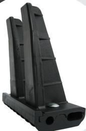
Weight saving and wear resistance are the keywords with the flights type KMP. This synthetic flight was especially designed to fulfil these two requirements. KMP flights are 160mm wide and available in 3 heights. These flights are in 2 parts and therefore they can be mounted very easy on existing sieve webs.
