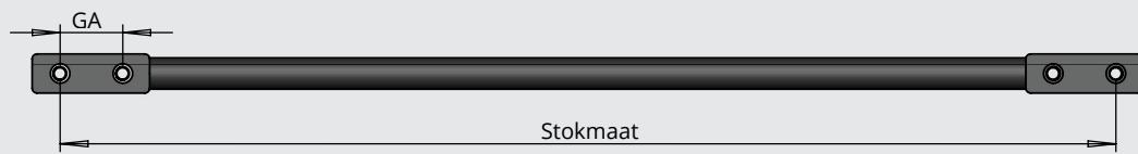
In determining the correct width of the sieve web, it is important that the rods have the correct "stokmaat". This is the distance between the two outside rivet holes, C.T.C. When ordering loose rods it is important that you mention the stokmaat as well as the distance between the holes in one end.
