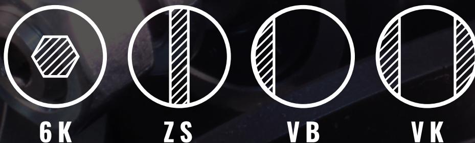
To make mounting easier, we generally supply the rollers with a threaded axle with a hexagonal hole (6K). Other possibilities are a saw cut (ZS), flat surface (VB) or a flat piece (VK) on the shoulder or on top of the axle.
