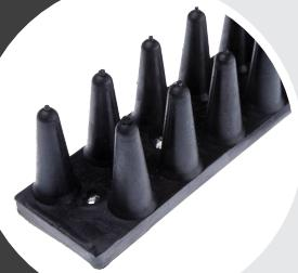
This is a flat steel profile, 4x30mm, on which 2 rows of rubber fingers are vulcanized. compared to the P30 profile the fingers are side shifted. These fingers are also 30mm high and placed C.T.C. 20mm from each other. D30 rods are usually riveted to traction belts with a pitch of 40mm.
